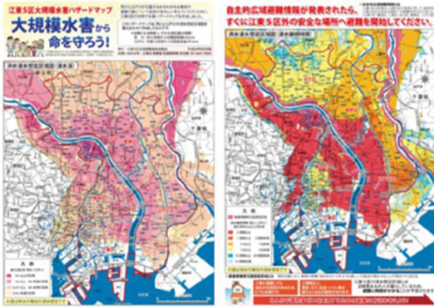
Example Hazard Map from Koto City that is a part of the east side of Tokyo, the left side shows inundation levels where deep red is over 5m depth due to tsunami or heavy rain, and the right shows time it would take for the water after a flood to disappear, and red is over two weeks time [ref2].
