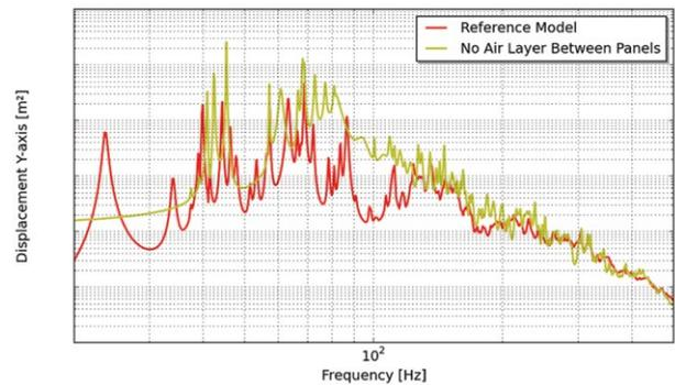
Figure 2. Solar Panels Vibration Spectrum, Impact of Air Interlayer Modeling
