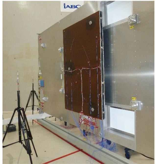
Figure 5. Reverberant Room Test Set-Up
