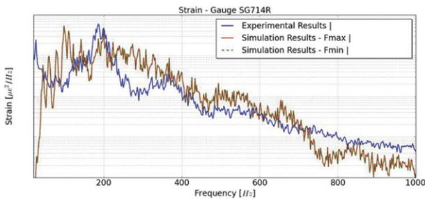
Figure 8. Solar Panel, Strain Power Spectrum
