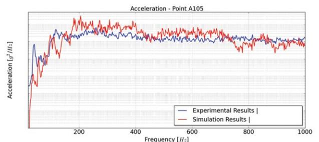
Figure 7. Solar Panel Acceleration Power Spectrum
