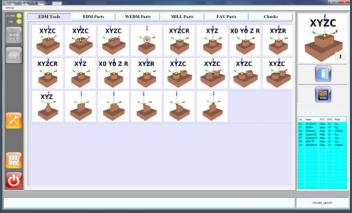
Guided Presetting of electrodes and workpieces, even on a pallet. With a single station, you can feed die-sinking and wire-cutting EDM machines and different milling centres.
