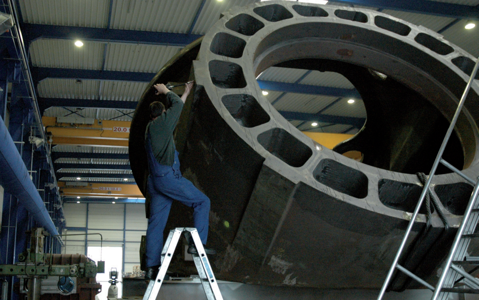
Measuring a BARD machine support.
