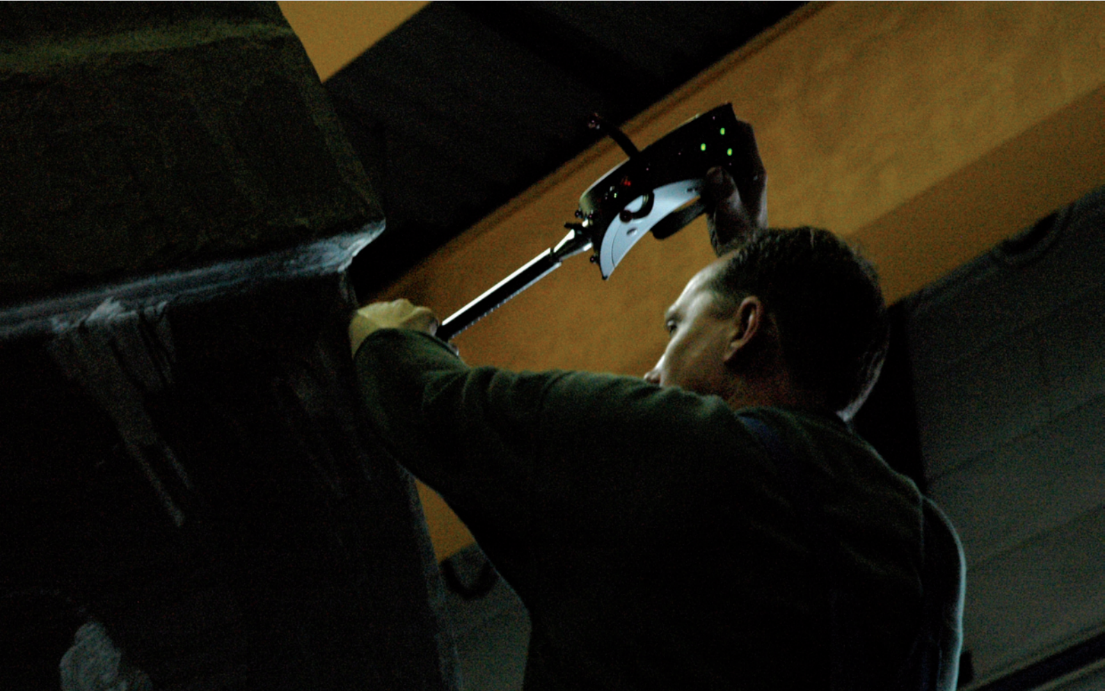
On top thanks to the Leica T-Probe: the mobile CMM makes it easy to measure points that are difficult to access.
