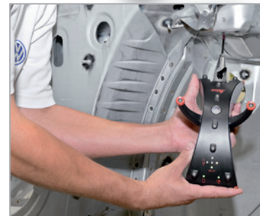
Wireless inspection of hidden points
